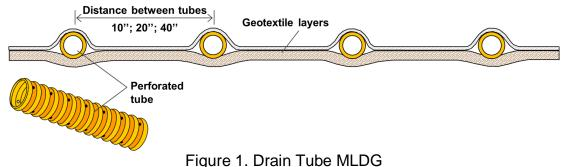
Drain Tube MLDG is unrolled directly on the lining system (figure 2) and connected down the slope to a collector trench or a ditch.
