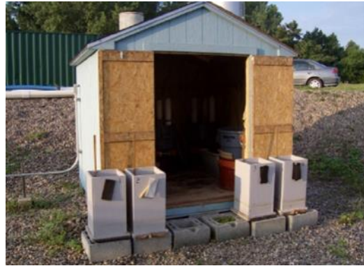
Figure 8 Field shed containing test columns
