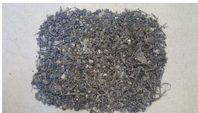
Figure 6: Picture of the coarser fraction (> 14 mm) of the RAP obtained when milling the section containing the geosynthetic. Some fibers/filaments are visible but represent less than 1% of the total weight of the RAP.
