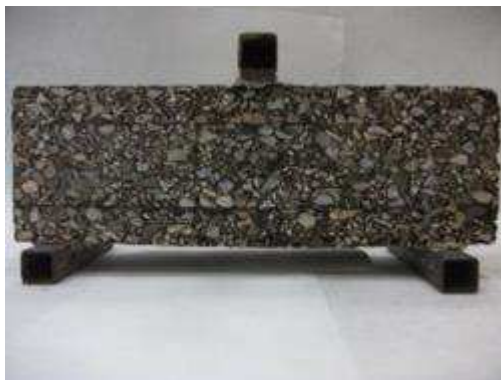
Figure 4: 100 x 75 x 300 mm 3 beams for the fatigue test of the AC reinforced with two layers of the coated geosynthetic combining fiberglass geogrid and light veil (GG/veil C 100x100).
