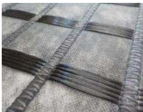
Figure 1: The geosynthetics described in this paper are obtained by warp-knitting a geotextile and a glass-fiber geogrid. An additional coating can also be added when needed (here, with bituminous coating).
