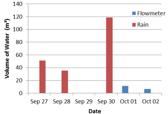
Figure 8. Volume of rain and water measured with the flowmeter surrounding the 10 year return period for a 12 hour rainfall event.
