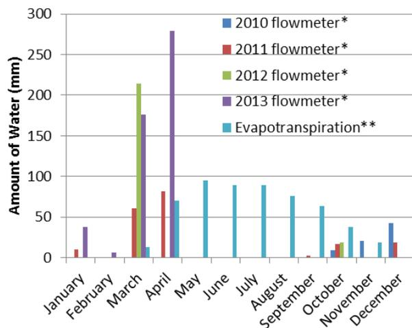
Figure 6. Comparison of 42-year average evapotranspiration, and amount of water calculated from monthly flowmeter volume. \*Flowmeter data is the volume of water collected in the geocomposite divided by the test pad area. \*\*Evapotranspiration data from Martin and Gray.
